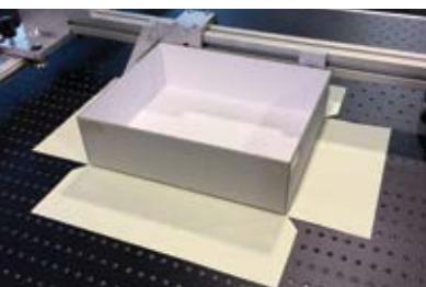
Guides for positioning the box and the board
